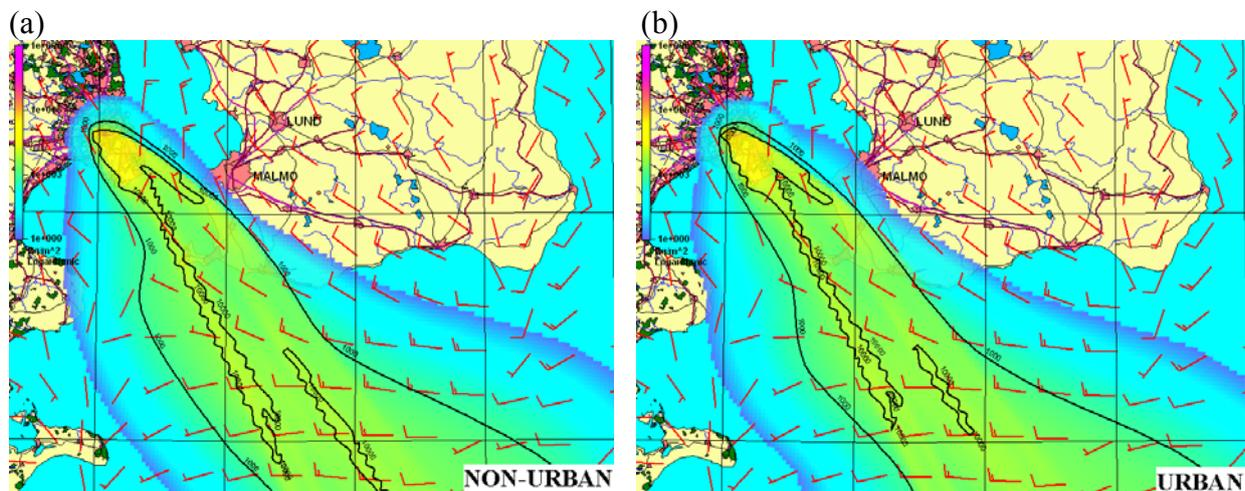
Fig. 4 – Total deposition patterns of  $^{137}\text{Cs}$  resulted from hypothetical accidental release in the Copenhagen metropolitan area /logarithmic scale ranging from 1 to  $1\text{e}+9$  Bq/m $^2$ /.
